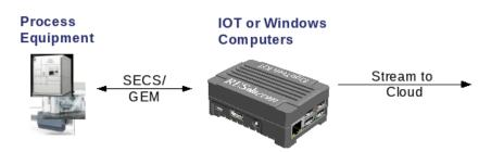
IOT concepts are relatively easy to understand. In a fab, tools usually communicate using SECS/GEM making the primary function of IOT to transmit SECS/GEM data to the Cloud. For data collection, some newer systems support "Interface A" an XML based stream protocol for data collection.
